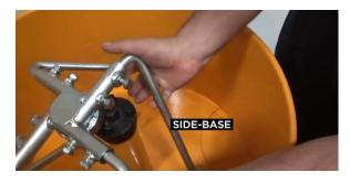
To mount the side-base arm lift up the cross joint.
