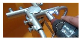
When the blade sits correctly, fasten the bolts - with spanner 16.
