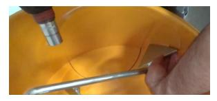
When the blade is 1-3 mm from the drum edge, fasten the bolts.
