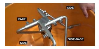
If you are changing all the arms, start with mounting the rake. Then mount a side arm on each side of the rake.
